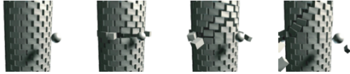
Figure 17: Test-cases that can reveal problems with freezing (sleeping policies). If too aggressive bricks will hang unnaturally in the air.
